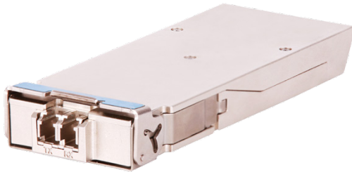
Figure 11 CFP2 transceiver module
